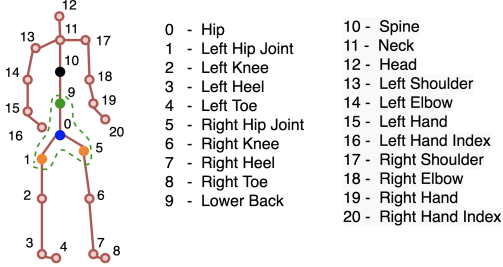
Fig. 2: The spatial graph of the human skeleton in this paper. Each node represents the body marker on the right [8].
